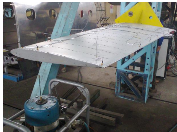
Figure 2. Configuration during testing with electrodynamic shaker
