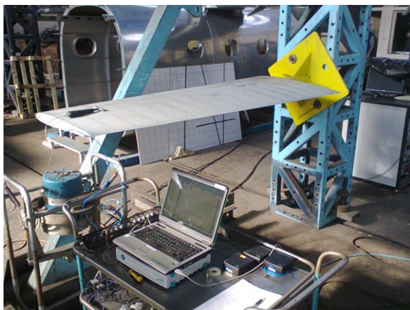
Figure 1. Mounting of the stabilizer in the test bench during impact hammer testing
