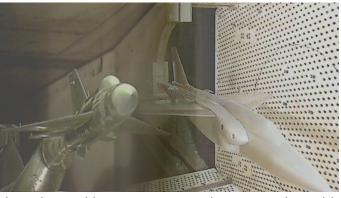
This facility has an interchangeable porous transonic test section with variable porosity from 0.01% up to 9% and 780 mm schlieren windows. State of the art data acquisition system and new investigation capabilities (CTS system and PIV) are under constant development. In this facility several important Romanian aeronautical projects have been performed, from military IAR-93 combat and IAR-99 trainer, air-to-air missiles and UAV systems, to civil aviation programs IAR-705 and ROMBAC (BAC 1-11).
