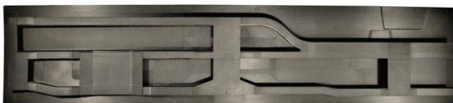
Figure 11: A320 NLGD manufactured by Coexpair (one-shot injection).
