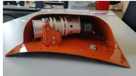
Figure 5: Camera position (top) and camera and fairing (bottom) on DLR ATRA A320. Courtesy of DLR.
