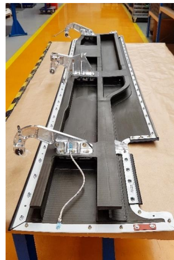
Figure 14: NLGD during fittings assembly at SSA.
