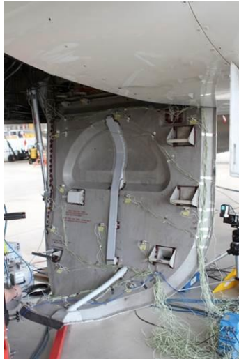
Fig. 11: Instrumented main landing gear door on the DLR ATRA A320 during the GVT.
