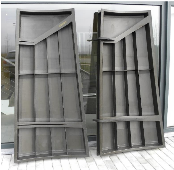
Fig. 19 : "I" stiffener panel doors manufactured by Coexpair & SLCA in European IMS&CPS FP7 project (= experience gained & manufacturing risks mitigated).
