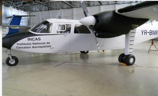
YR – BNR / YR – BNM / YR - BNN Britten Norman BN-2A-21 Flying labs – Radar & EOS surveillance
