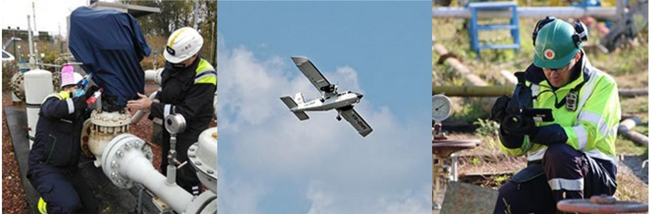
*Leak quantification with High Flow Sampler    INCAS' aircraft to capture methane leaks    Screening with IR camera by The Sniffers by The Sniffers*
